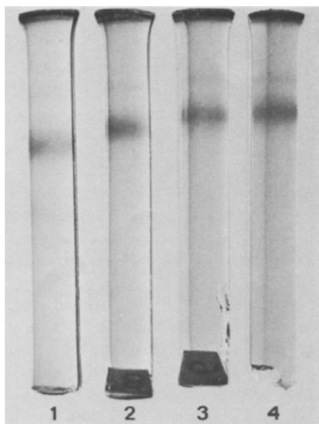
Fig. 5. Affinity electrophoresis of pea \alpha -D-galactosidase II. 1 = Control gel; 2-4 = affinity gels containing O- \alpha -D-galactosylpolyacrylamide copolymer (concentration of immobilized sugar, c_i = 1.0 \cdot 10^{-3} , 2.0 \cdot 10^{-3} and 2.5 \cdot 10^{-3} M, respectively).
